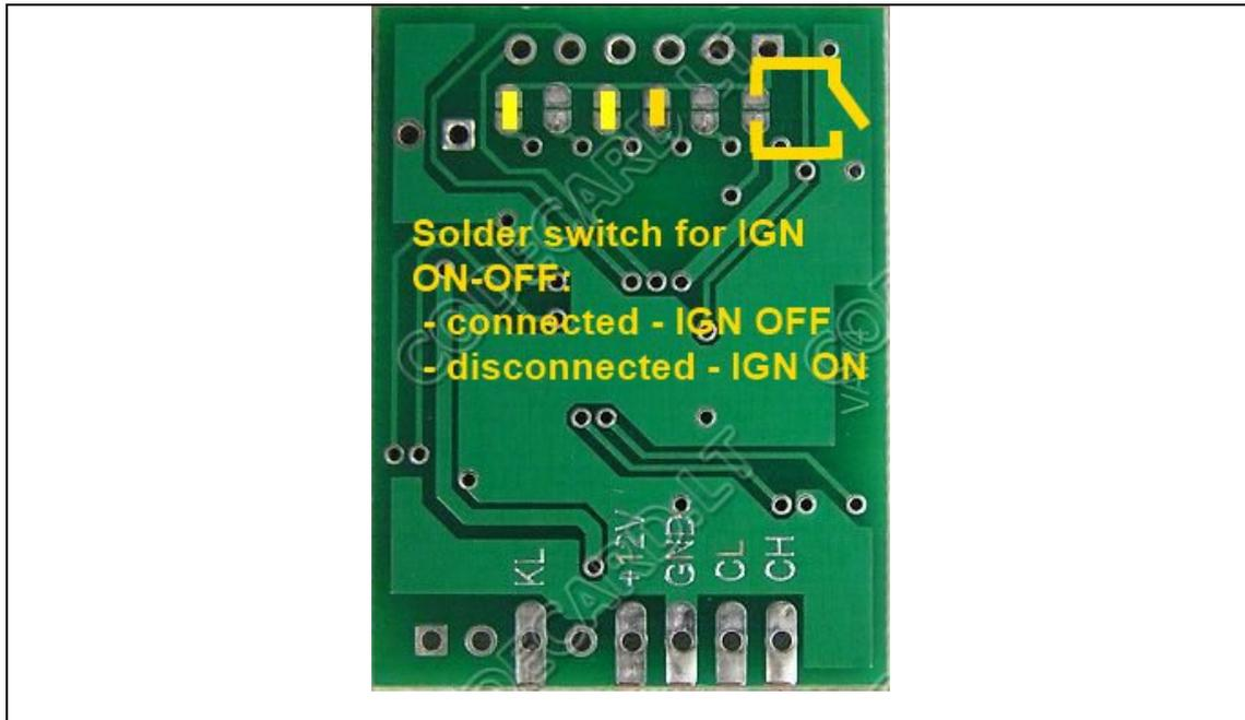
Audi dash with grey connector emulator connection pinout:
